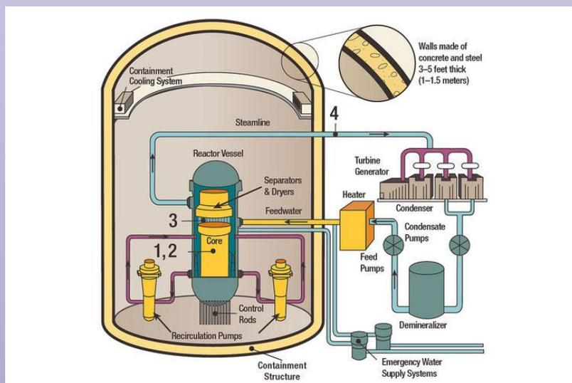
A diagram of a boiling water reactor.
