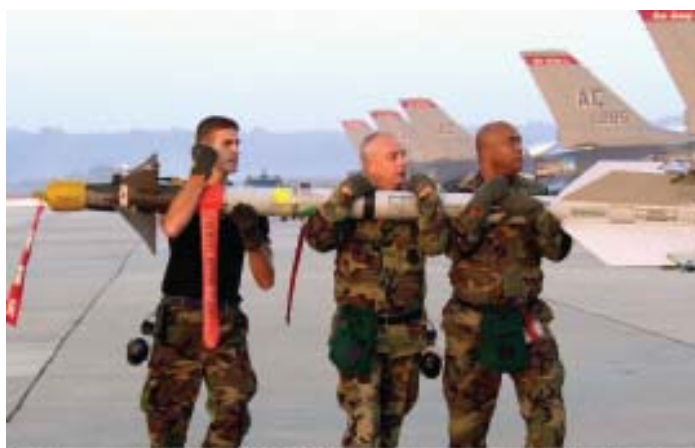
Weapons load team (l-r) Senior Airman James Keefer, Master Sgt. Frank Buzby and Tech. Sgt. Wendell Hunte load an AIM-9 on a 177th Fighter Wing F-16C. Photo by Master Sgt. Don Taggart, 177FW/SVSC.
