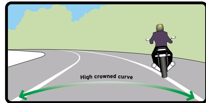
The only way to handle the wrong-way banking is to slow down. This will straighten the motorcycle and reduce the outward force.
