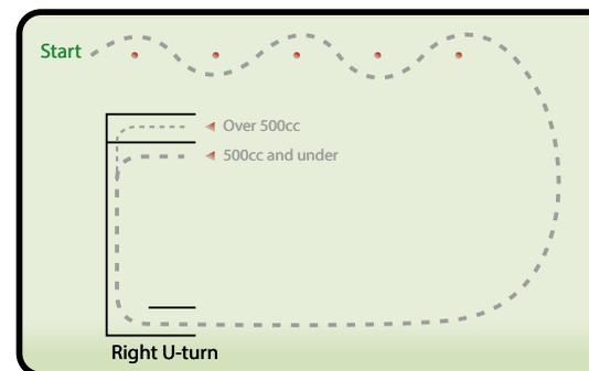
The examiner will evaluate an applicant's ability to stay within the path of travel without touching lines or cones, and without putting a foot down. Cones are 12 feet apart with a two-foot offset.
