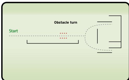
**4. Obstacle Swerve:** Tests an applicant's ability to swerve the motorcycle quickly to avoid an obstacle. An applicant will be evaluated on the ability to stay within the path of travel and turn quickly without touching a boundary line.
