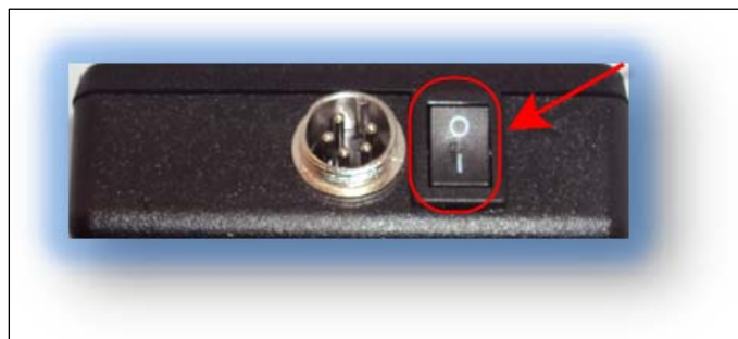
Figure 5-3: Scan Tach Power Switch in ON position
