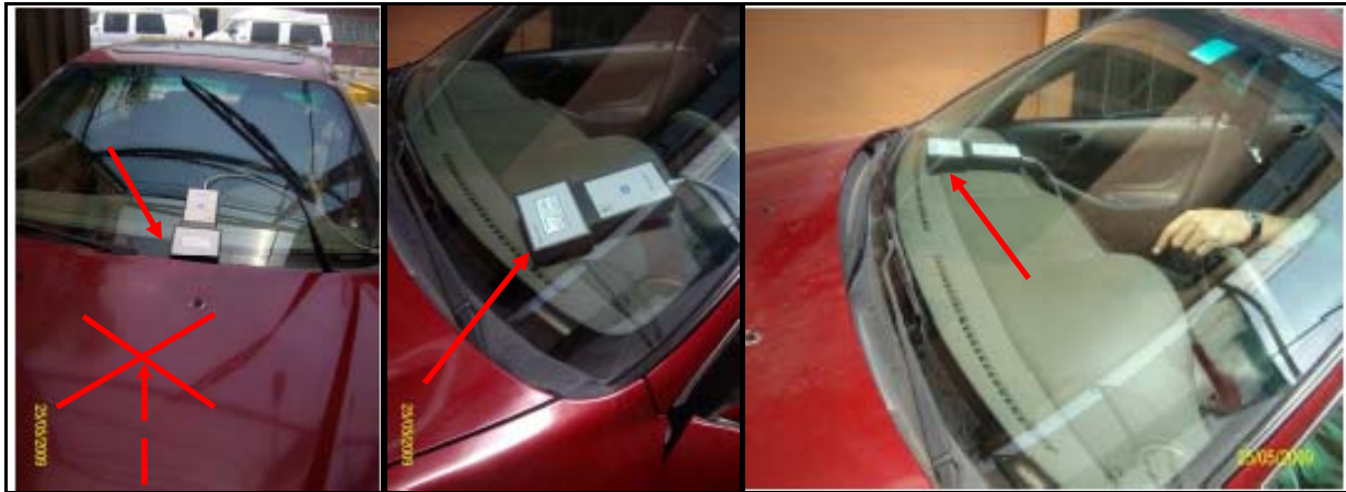
Figure 5-5: Sample Locations for Obtaining RPM Readings
