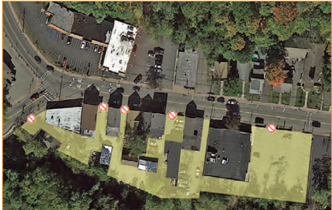
Currently, these ten properties have separate private parking lots and seven driveways interrupting pedestrian flow along Main Street. This example shows how separate existing parking areas could be shared to reduce the number of driveways from seven down to two, while providing 45,500 square feet of space to accommodate about 165 vehicles. Employee parking could be designated as needed, and some of that space should be dedicated to a greenway along the river.
