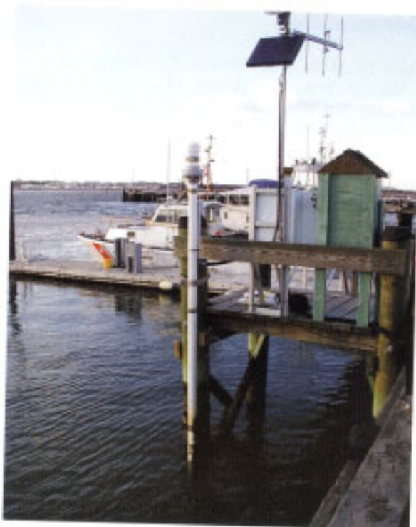
Figure 4. U.S. Geological Survey tide gage at Cape May Harbor in Cape May, N.J., which transmits tide elevation and meteorologic data via satellite and VHF radio for emergency management and other purposes. (Photograph by Peter B. Reilly, U.S. Geological Survey)
