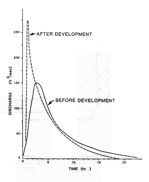
Fig. 3. Comparison of unit-hydrographs of a Pinelands subwatershed (portion of the Upper Great Egg Harbor River) before and after development. The hydrographs are for high intensity/short duration storms. Note that urbanization results in increased peak discharge (redrawn from, Fusillo 1981).
