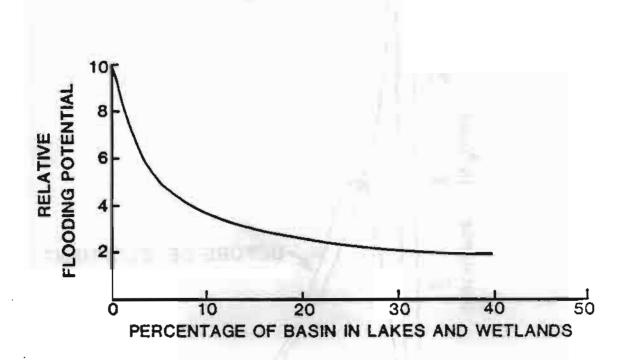
Fig. 2. Relative flooding potential in basins with different percentages of lakes and wetlands. Curve is based on data from Wisconsin watersheds. Note the significant increase in the potential for flooding in basins with a low percentage of lakes and wetlands (redrawn from, Novitzki 1979).
