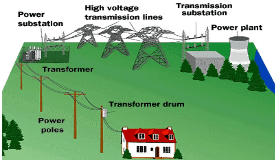
The power flowing down high-voltage lines is between 155,000 to 765,000 volts. That amount of power is unsuitable for data transmission. It's too "noisy." Both electricity and the RF used to transmit data vibrate at certain frequencies. In order for data to transmit cleanly from point to point, it must have a dedicated band of the radio spectrum at which to vibrate without interference from other sources.
