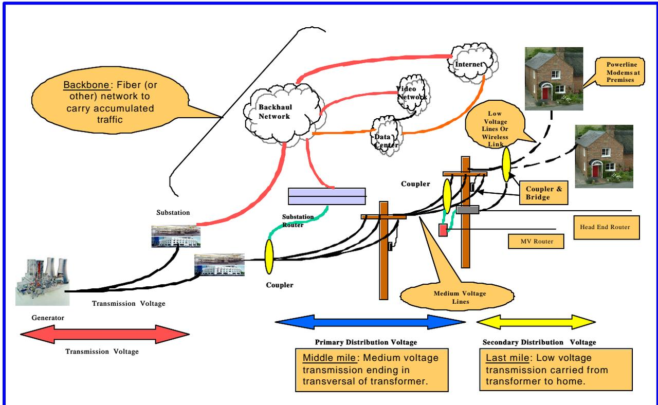
By combining the technological principles of radio, wireless networking, and modems, developers have created a way to send data over power lines and into homes at speeds equivalent to those of DSL and cable. By modifying the current power grids with specialized equipment, the BPL developers could partner with power companies and Internet service providers (ISPs) to bring broadband to everyone with access to electricity.
