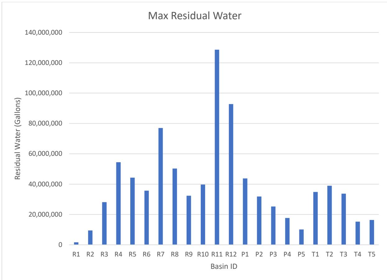
Figure 33. The Route 9 corridor has the basins with the most residual water. Of these, R11 and R12 produce substantially more than any other basin. To reduce total residual water for the township, these basins must have adjustments. Basins R4 and R7 are also important to focus on.
