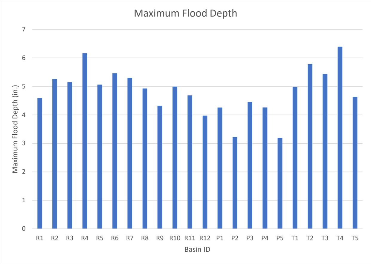
Figure 34. Summary of the flood depths for the individual basins. These flood depths are the maximum that occur during any storm interval and distribution.
