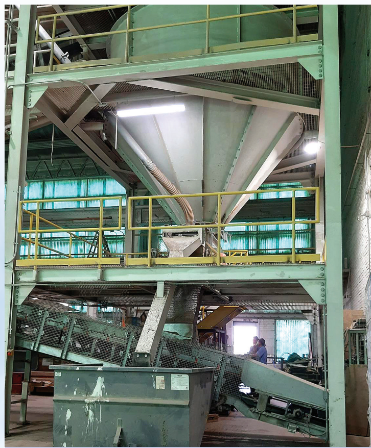
Pictured: The manufacturing process takes 100% curbside recycled glass powder and mixes it with a foaming agent.
