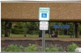
AFTER: on 7/30/10 the van accessible space was restriped to make it larger. A sign was installed at van space reading "Van Accessible". Additionally, a Truncated Dome was added to the existing curb ramp on 9/3/10.
