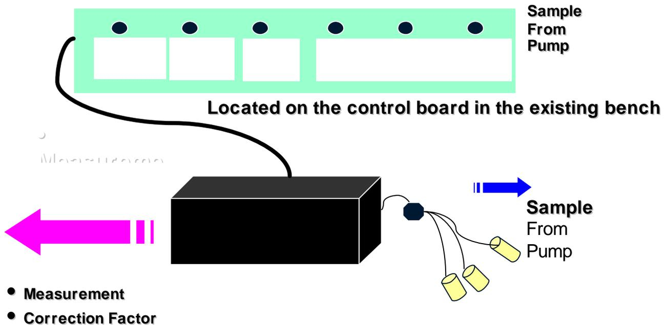
The wide response sensors were interfaced to an electronic system that conditions the input signals, improves signal-to-noise ratio, and employs a pattern recognition algorithm to determine to which volatile chemical the set of sensors are exposed.
