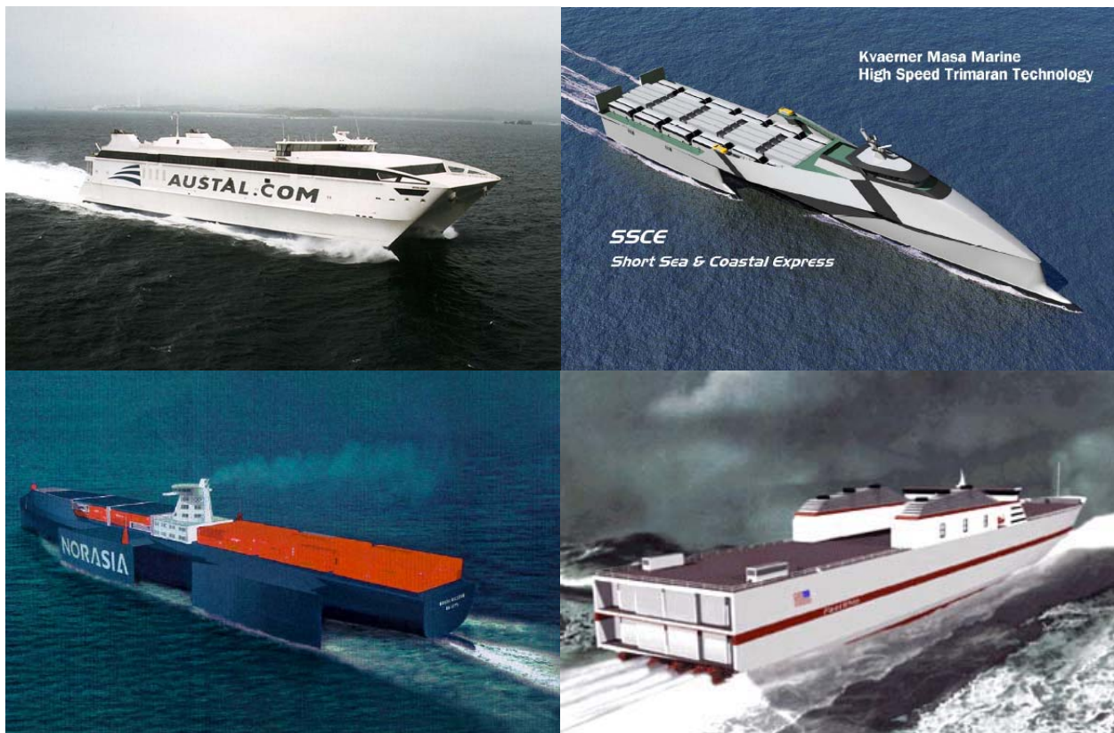
Figure 19. Fast Freight Ferry Technologies 19-1 (top left) West Pac Express vessel currently being built by the Austal for U.S. Army 19-2 (top right) Ro-Ro and container trimaran vessel designed by Kvaerner Masa-Yards 19-3 (bottom left) Ro-Ro and container pentamaran vessel designed by Kvaerner Masa-Yards 19-4 (bottom right) FastShip Atlantic vessel
