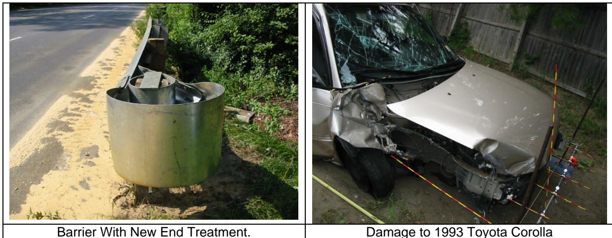
Figure 9. Replaced Guide Rail End Treatment and Damage to 1993 Toyota Corolla
