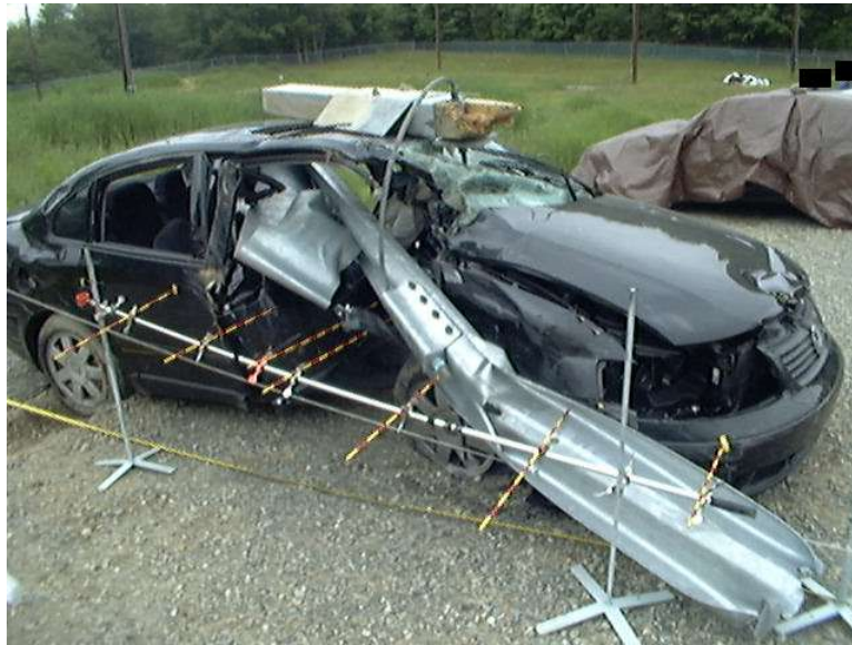
Figure 1. Collisions with Guide rail are not always forgiving. [NASS/CDS Case 2001-81-036 - Fatal Side Impact of 1999 VW Passat into Guide Rail End Treatment ]
