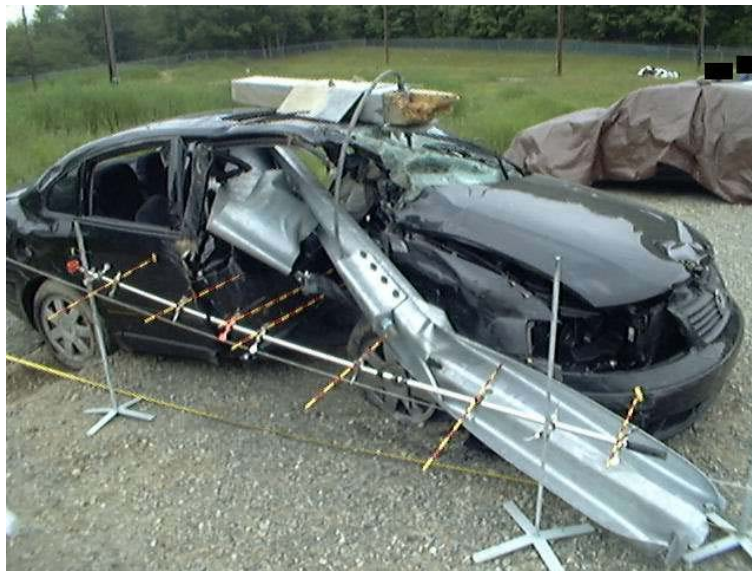
Figure 15. Guide Rail End treatments are not designed for Side Impact [NASS/CDS Case 2001-81-036]
