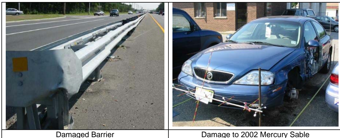
Figure 8. Barrier and Vehicle Damage in 2002 Mercury Sable – End Treatment Collision
