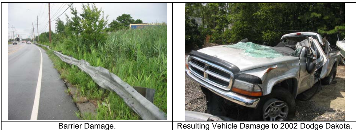
Figure 12. Barrier and Vehicle Damage in 2002 Dodge Dakota – Guide Rail Collision
