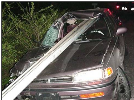
Figure 3. Poor End Terminal Performance: Vehicle Spearing
