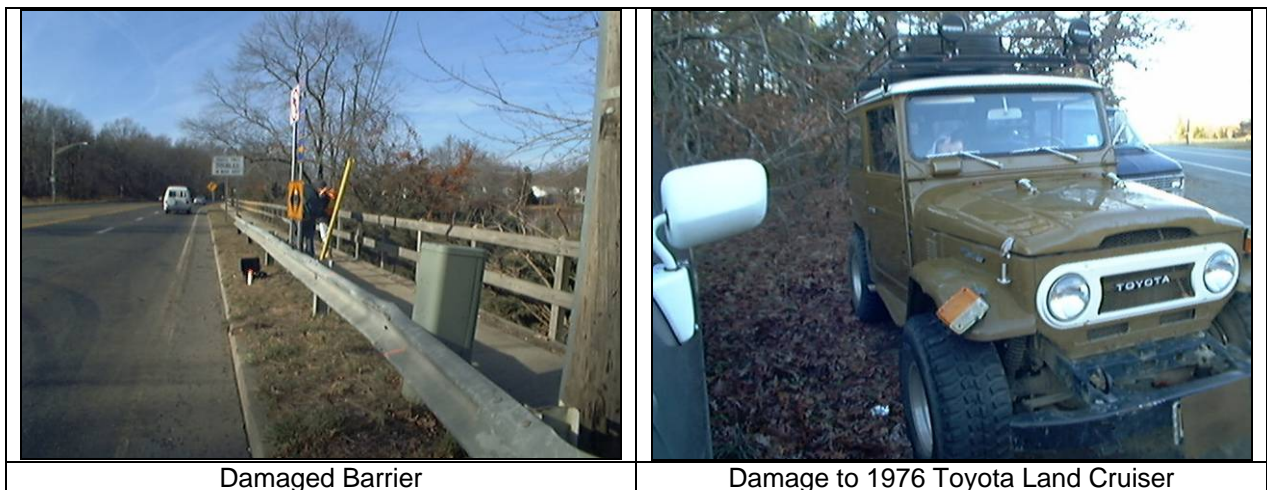
Figure 21. Barrier and Vehicle Damage in 1976 Toyota Land Cruiser – Guide Rail Collision
