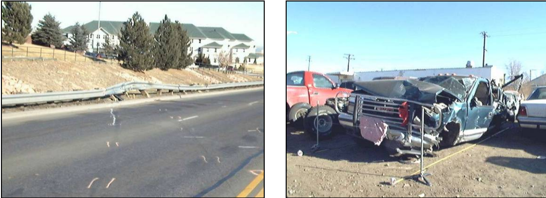
Figure 11. Higher Center-of-Gravity SUVs can “vault” a guide rail system. In this 2001 case, a 1992 GMC Suburban became airborne on impact with a W-beam guide rail, overturned, and injured the driver. (Ref: NASS/CDS 2001-75-001)
