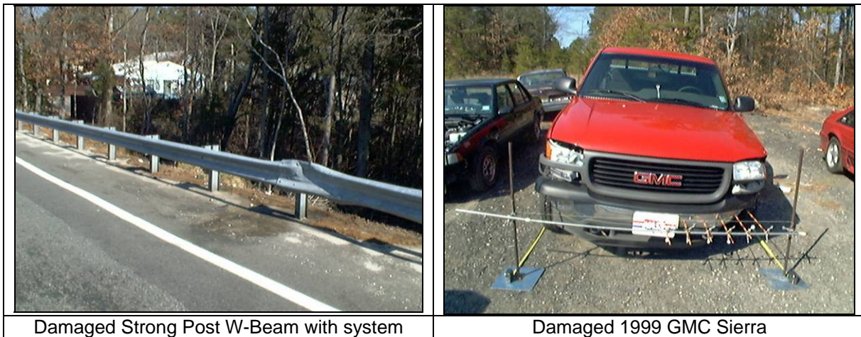
Figure 16. Barrier and Vehicle Damage in 1999 GMC Sierra – Guide Rail Collision
