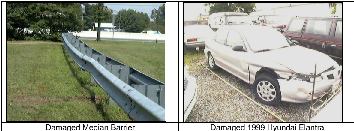
Figure 19. Barrier and Vehicle Damage in 1999 Hyundai Elantra – Median Barrier Collision
