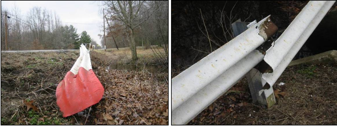
Figure 29. View of Damaged End Terminal (Left) and Failed Splice Location (Right)
