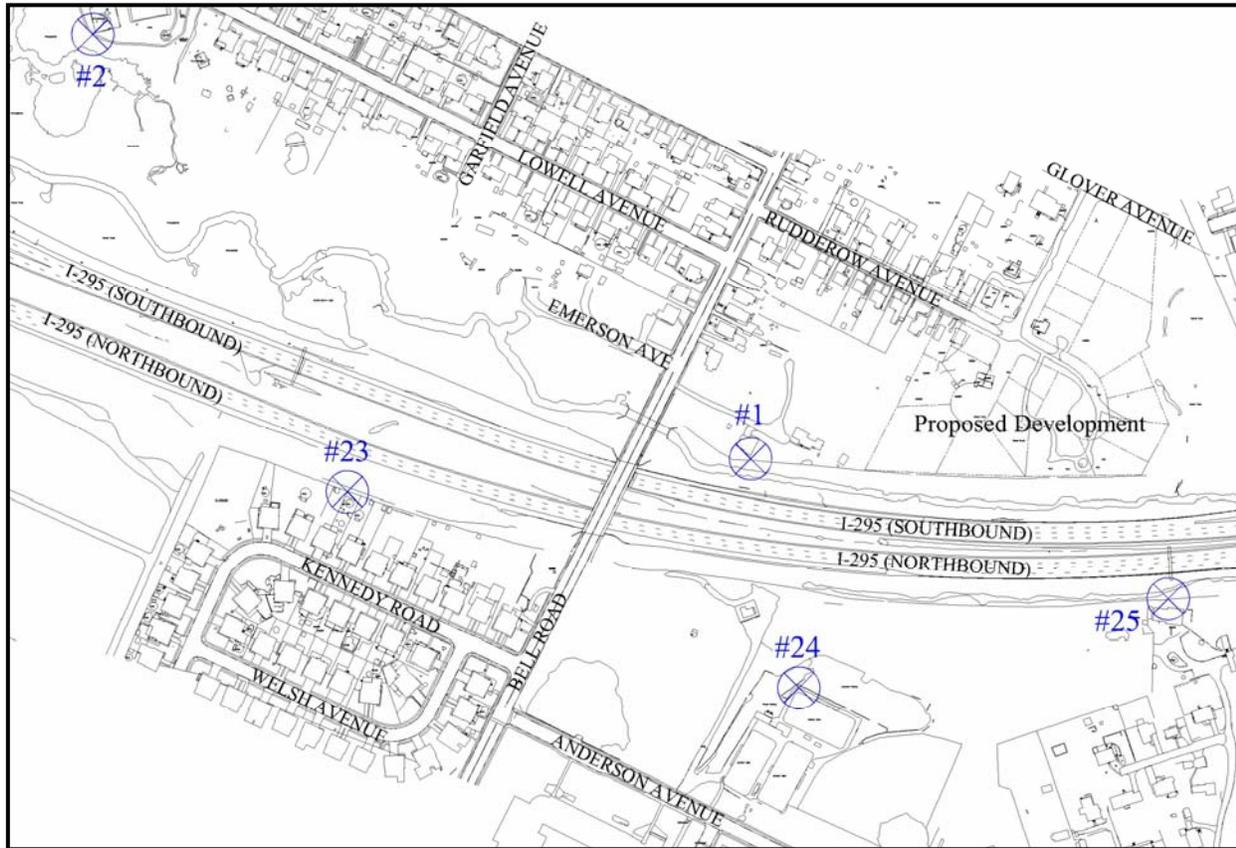
Receptor #1 is located along the I-295 southbound right-of-way line, representing the neighborhoods near Bell Road as well as Lowell, Emerson and Rudderow Avenues. Receptor #23 and Receptor #25 are located along the I-295 northbound right-of-way line, representing the neighborhoods near Bell Road, Kennedy Road and Anderson Avenue. Receptor #2 represents the Shining Star Park, while Receptor #24 represents the Scott E. Mueller Park.
