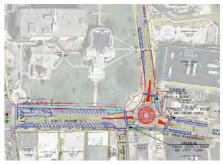
**Route 28 (Main Street) Safety Improvements** This section of Somerville (NJ) Borough's Main Street is a primary traffic corridor with heavy pedestrian use in this County seat. STV's conceptual plans include ADA-compliant curb ramps, push buttons, and pedestrian countdown heads; improved lighting; an upgraded traffic signal with a lead pedestrian interval, and a potential roundabout.
