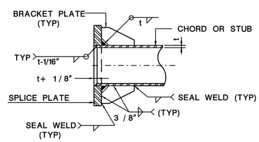
**CHORD SPLICE ASSEMBLY WELD DETAIL**
