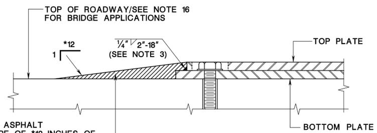
**SECTION: B-B FOR LOW SPEED INSTALLATION (<= 45 MPH)**
