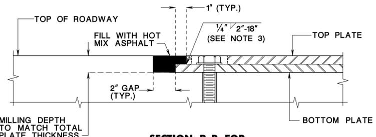
**SECTION: B-B FOR HIGH SPEED INSTALLATION (> 45 MPH)**
