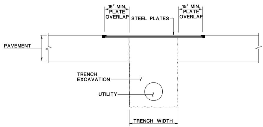
**SECTION: A-A FOR HIGH SPEED INSTALLATION (> 45 MPH)**
