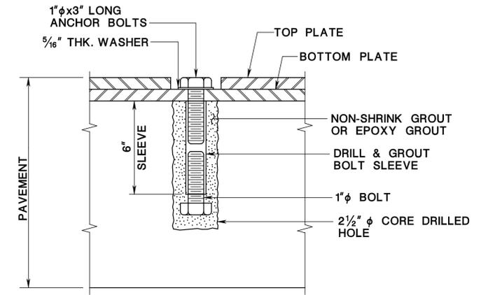
**STEEL PLATE ANCHORING DETAIL**
