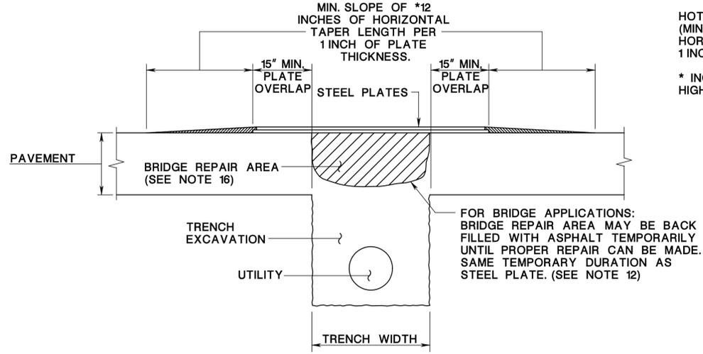
**SECTION: A-A FOR LOW SPEED INSTALLATION (<= 45 MPH)**
