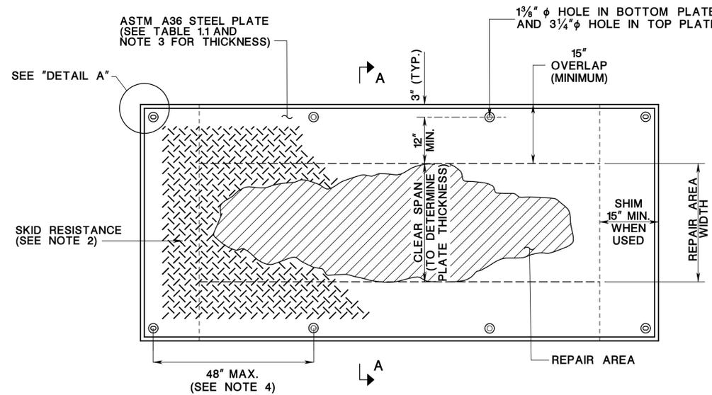
**PLAN - STEEL PLATE OVER REPAIR AREA**
