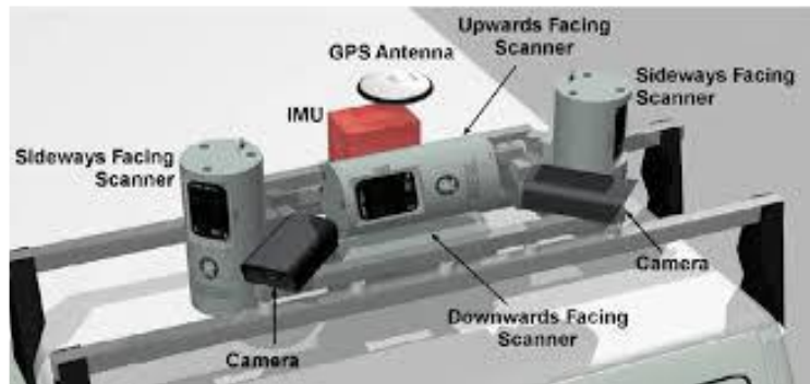
Depiction of Various Mobile LiDAR Equipment Mounted on Vehicle
