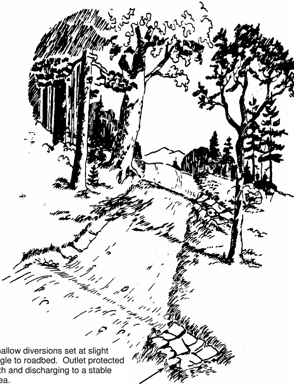
Shallow diversions set at slight angle to roadbed. Outlet protected with and discharging to a stable area.
