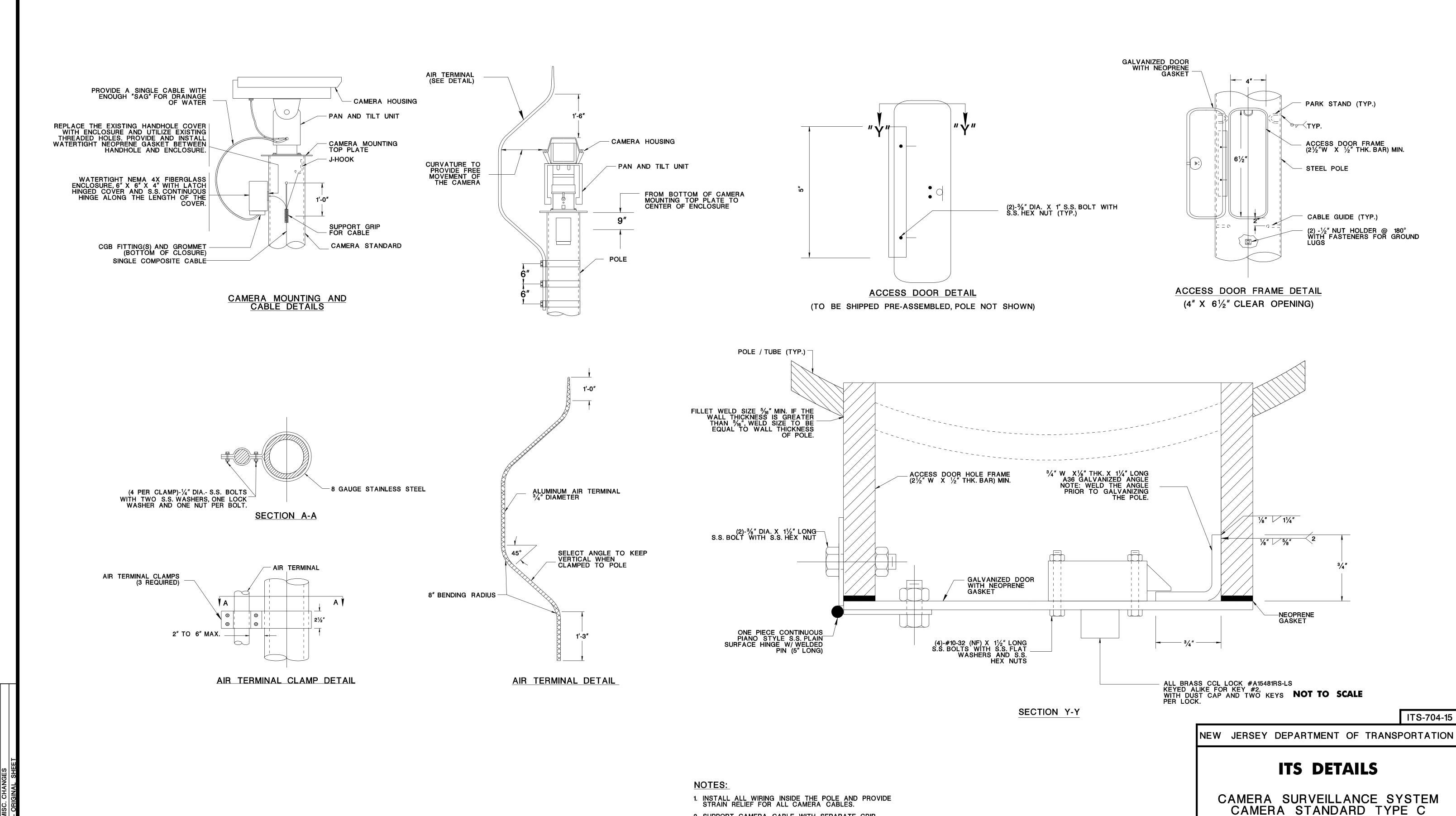
2. SUPPORT CAMERA CABLE WITH SEPARATE GRIP.
