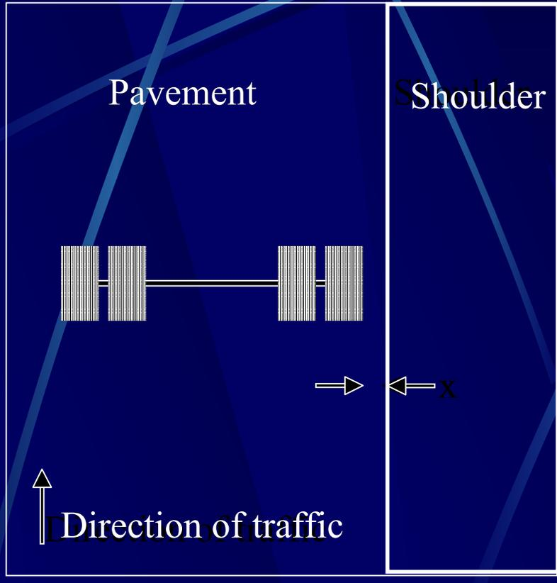
Used to calculate pavement responses & the number of axle load applications over a point for predicting distress & performance.
