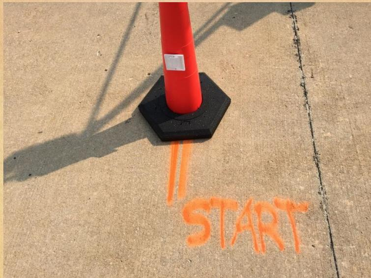
Place the reflectors on the edge of the road, a safe distance from the fog line/lane edge. Make sure the reflector is mounted to the cone at the correct height from the ground for the photocell to be triggered by the reflector.
