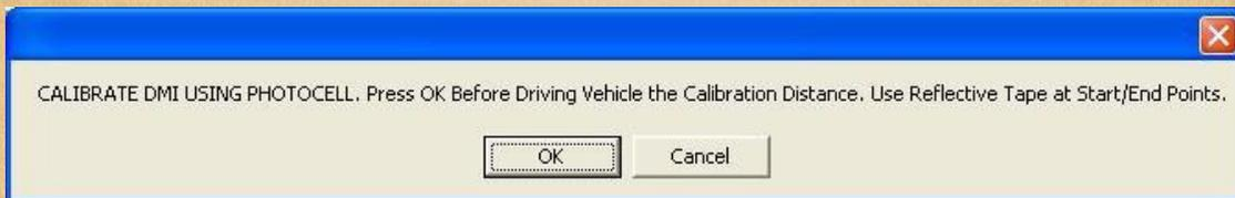
After the user clicks "OK", a timer will start. The user will have 300 seconds to complete the calibration process. Once the driver travels past the first reflector, the system will give an audible alert "START". If this alert is not given, the system has not been triggered successfully and will need to be checked.
