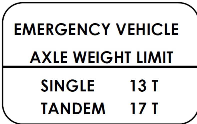
If a State law allows or exempts emergency vehicles to operate without restriction off the Interstate System as legal loads, 23 CFR 650.313(c) requires bridges on these highways to be load rated and posted, if necessary, for these vehicles. Unless State law relies on a different definition of emergency vehicle than that included in the FAST Act (23 U.S.C. 127(r)(2)), States can perform load ratings on these highways using the two emergency vehicle configurations included in this memorandum.
