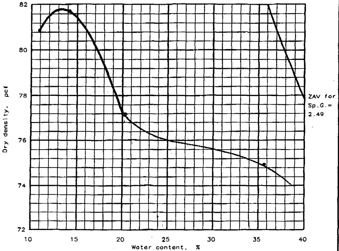
Test specification: ASTM D 1557-91 Procedure A, Modified
