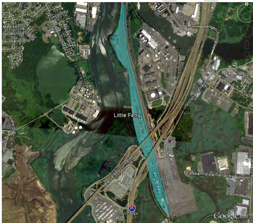
Figure 2-24: Little Ferry Intermodal Terminal Footprint
