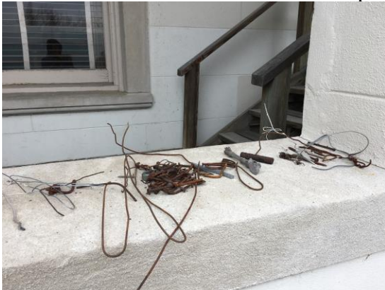
Metal debris found in the ballast
