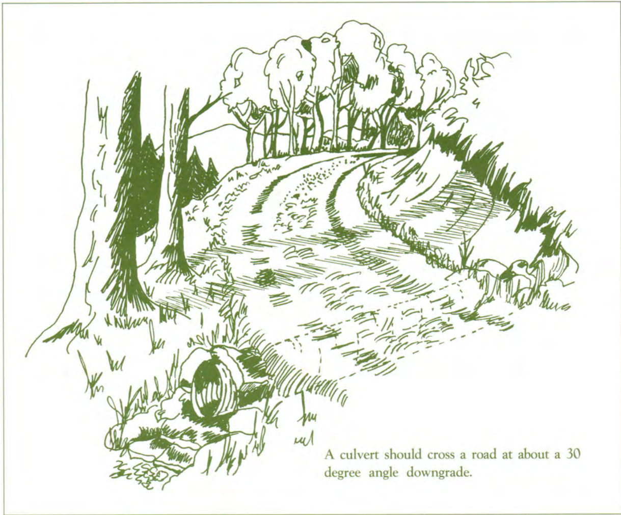
FIGURE 3 CULVERT INSTALLATION (GEORGIA FORESTRY COMMISSION 1988)
